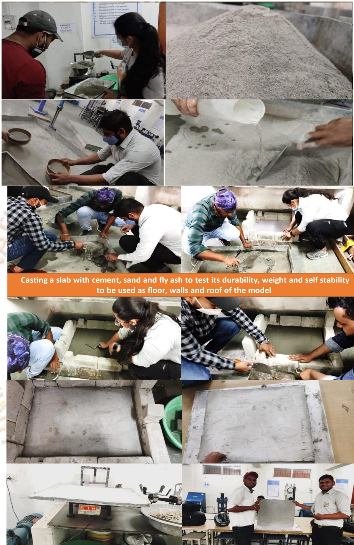
Fig 11 Slab Casting with Fly ash, sand, and cement
